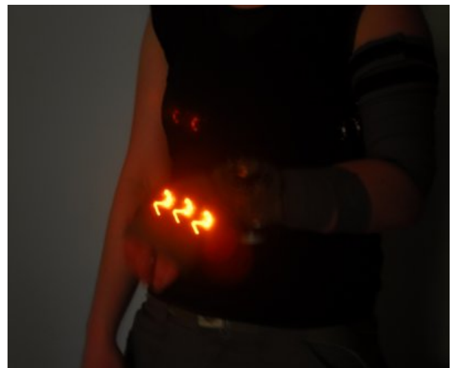
Figure 4. The Impact prototype by Catherine Marchand. As she starts to throw punches in the air, the red LEDs on the knuckles begin to glow.
